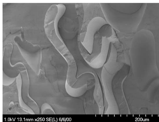
Fig. 5. Folding and incipient phase encapsulation associated with chaotic advection in a sample with 20% PS and N = 6 .
